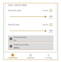
**Power-On level:** this is the intensity value to which the output is brought as soon as the device is powered.
